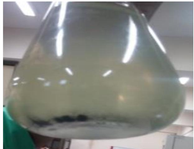
Figure: 7 Nano particle settlement after (2 hours)
