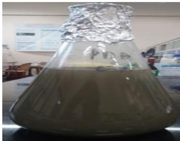
Figure: 11 Nano particle settlement after 10 hours
