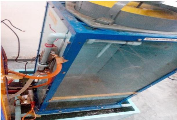
Figure: 15 Plate type Heat Exchanger
